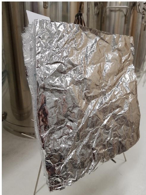
Polynum Reflective Insulation, aluminium foil in four layers and polyester in three layers
