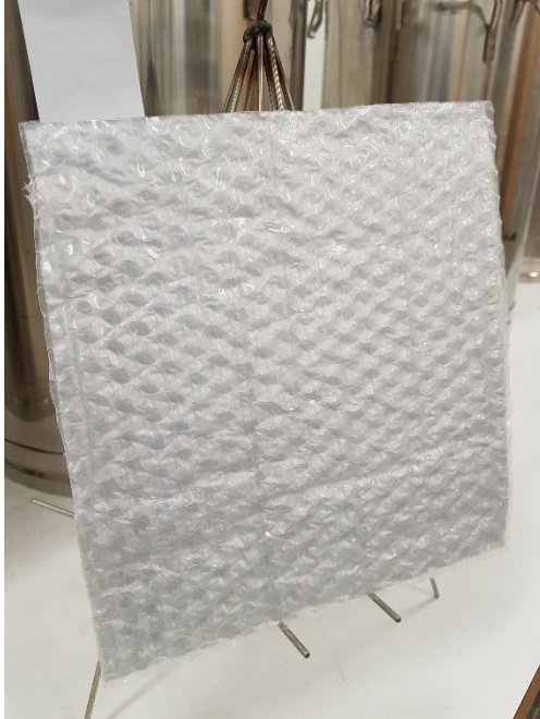
Polynum Reflective Insulation, bubble plastic – aluminium foil – bubble plastic
